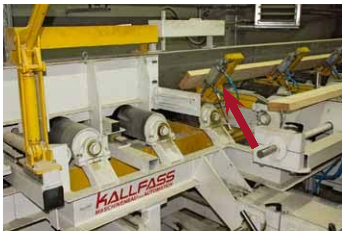
Longitudinal infeed into the band resaw with fixation for vertical lamellas
